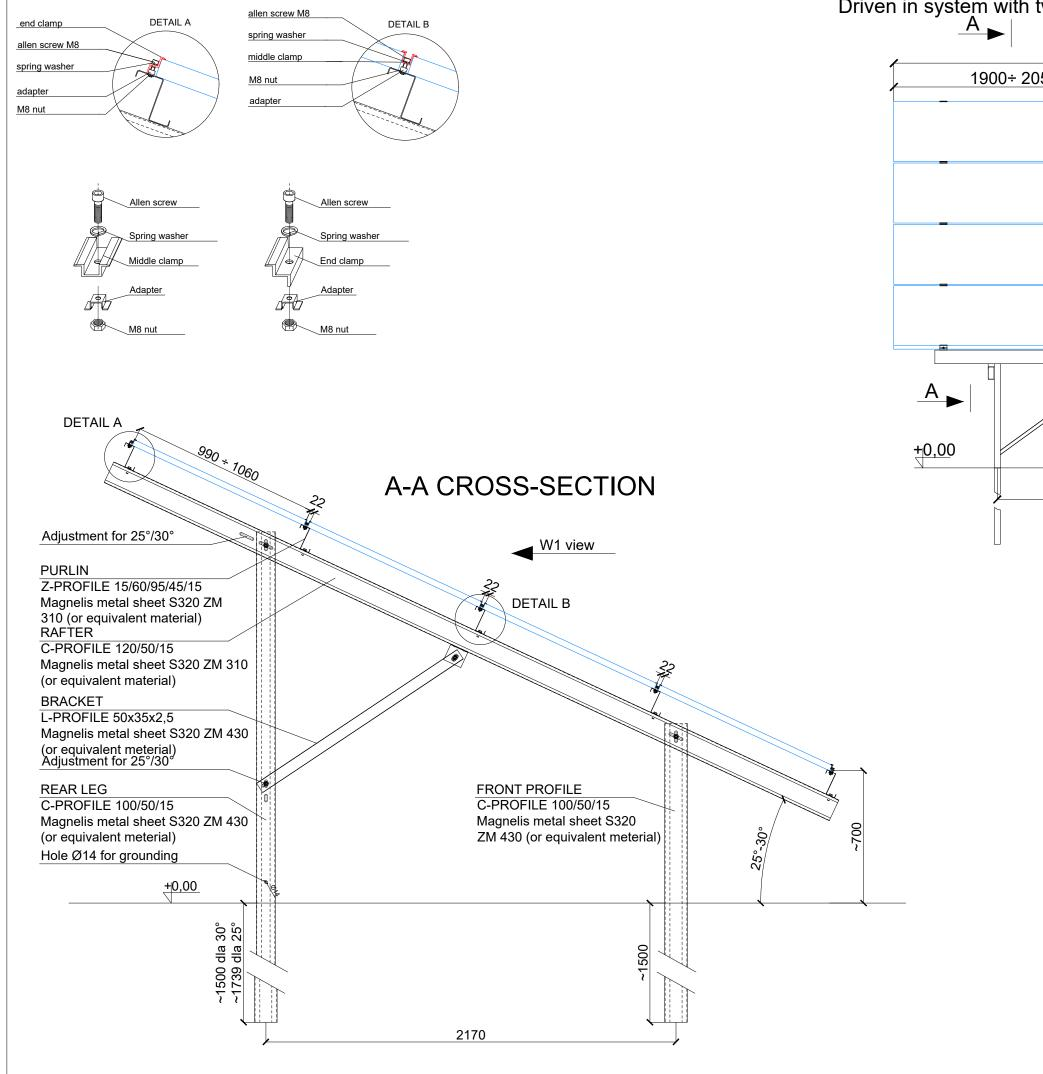
Driven in system with two supports, horizontal layout of modules
